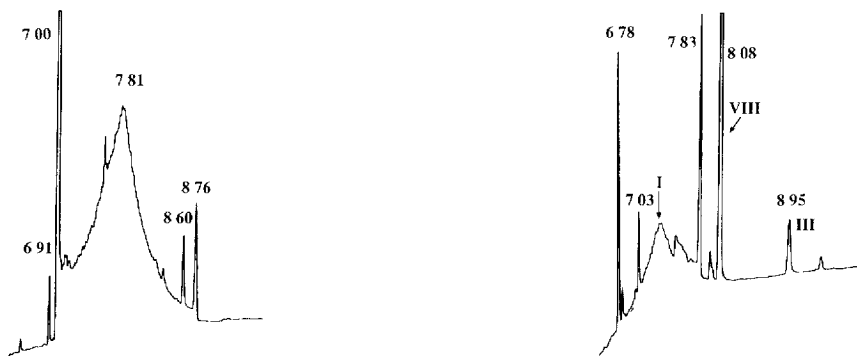
Fig. 3 Gas chromatogram of a pure solution containing compound I at a concentration of 10 ng/ \mu l demonstrating decomposition. Splitless injection mode, for GC conditions, see Capillary gas chromatography , chart speed, 2 cm/min. The numbers above the peaks indicate the retention times of the compounds.
